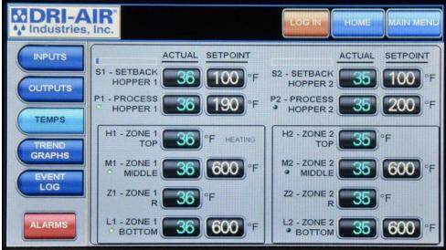
The temps screen is used to display all of the thermocouple temperatures to trouble shoot a problem. The current status of the regeneration cycle is displayed in the lower right of the display. We will use this screen while assisting in determining where to look to solve a problem. Heater outputs are also displayed by a small LED to the left of each heater's temperature readout.
