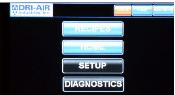
To enter the setup screen, first tap the main menu button in the top right of the touch screen, then select the "SETUP" button.
