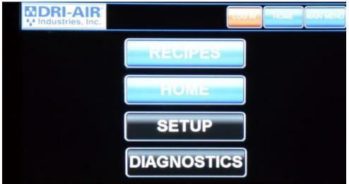
To enter the diagnostics screen, first tap the main menu button in the top right of the touch screen, and then select the "DIAGNOSTICS" button.
